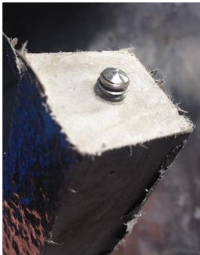
Cement paste prism for shrinkage measurement containing cellulose fibre.
