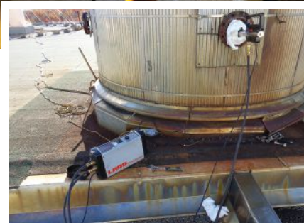
Acid dew point measurement on a recovery and biomass boiler stack.
