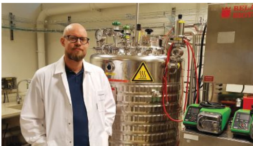
Björn Alriksson with one of Processum's bioreactors, which will produce bacterial nanocellulose.
