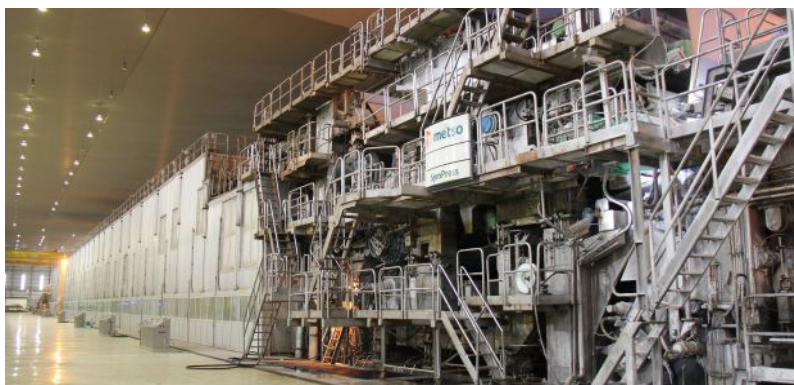
The mill's Paper Machine 3 (PM3) has a target running speed of 1,350 metres per minute and an average uptime operating efficiency of 85 to 90 per cent.
