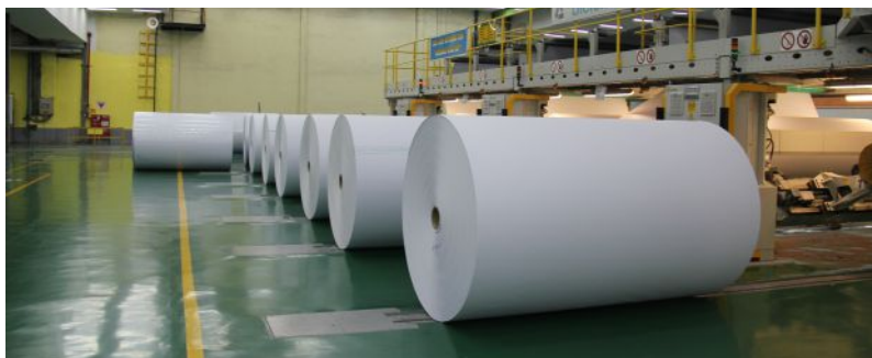
The Bielomatik-driven converting plant cuts jumbo rolls – 50-tonne paper rolls – into photocopy paper.
