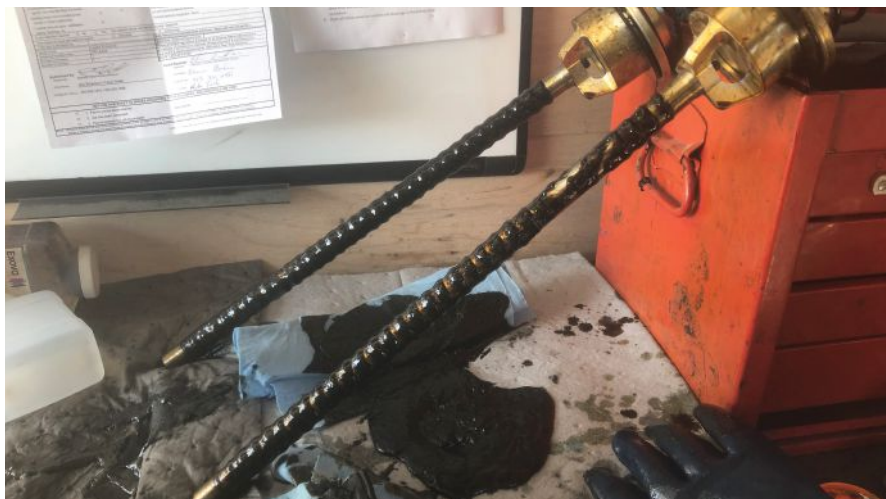
Rotor-Tech's 10- and 25-micron filters during mid-filtration inspection.
