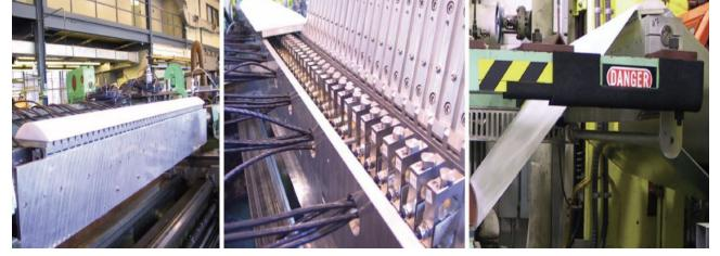
Figure 2: The tension beam installed on the lathe during its fabrication (left), inside view of the 50 load cells (centre) and the beam in operation with paper on it (right) [1].
